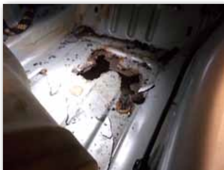
The extent of the floor damage on the offside, only really identified after removal of the carpets.
