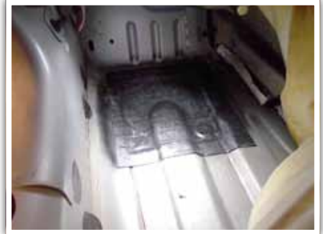
Repaired floorpan area with new sound deadening applied.
