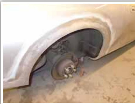
Later repair work on the wheelarch, before painting.
