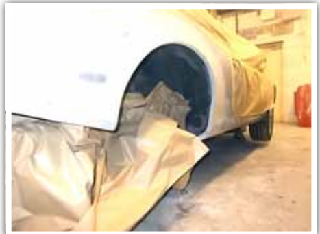
The offside prepared ready for painting.
