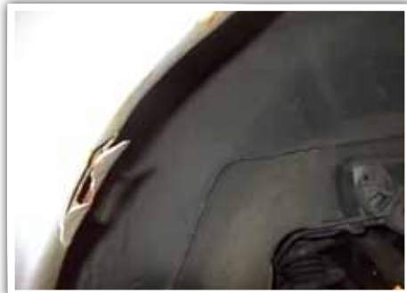
A typical example of wheelarch corrosion that has eaten its way through the bodywork.
