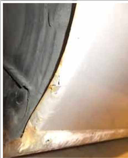
Rust breaking through not only the wheelarch but also the sill area.
