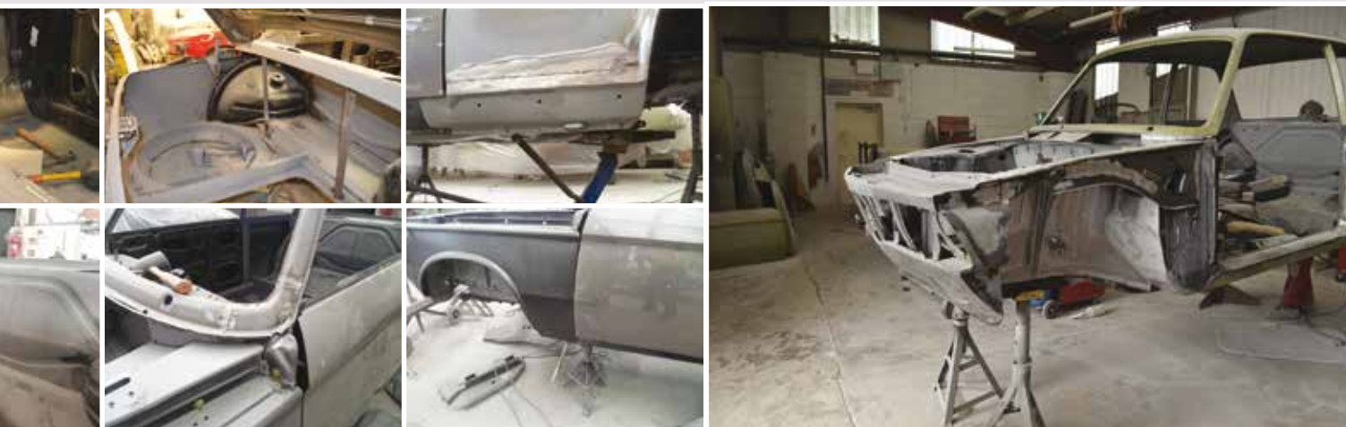
The car was sandblasted to remove all paint, primer, rust and crud! Once all trace of rust had been removed, David and his team then set about cutting out and repairing bodywork where necessary, raking out all joints, removing rust, running lead and then resealing, using bodyfiller on certain panels where needed, 'stitching' in repair panels if a large area needed replacing and welding into place lots of new body panels like the sills, wings etc – a laborious task...
