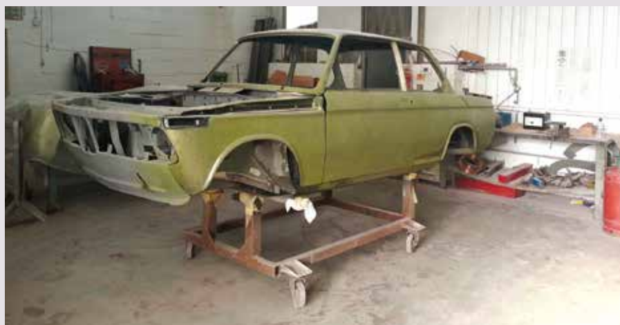
Getting there; my tii is nearly at the stage where it moves to the paint shop, it's already had a first coat of primer in places (the green-ish coating), just waiting for the bonnet to be fitted so the front end can be primered – then into the spray booth and the 2002 received its 2K Primer coat...
